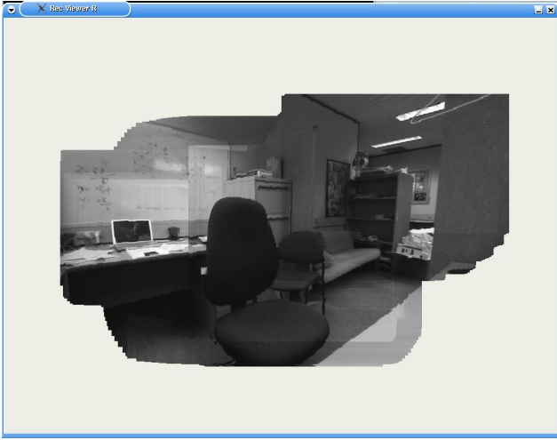
Figure 7: Online output of the active rectification process: mosaic of rectified frames from right CeDAR camera.
