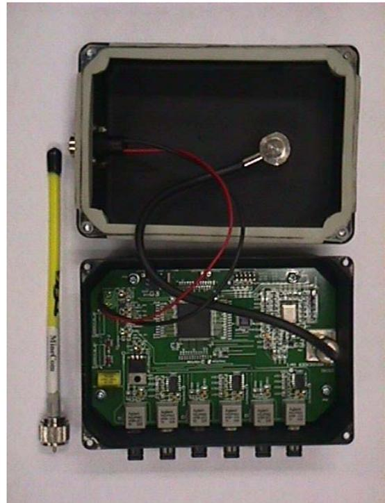
Fig. 9. Internal view of the LAMPS reader.
