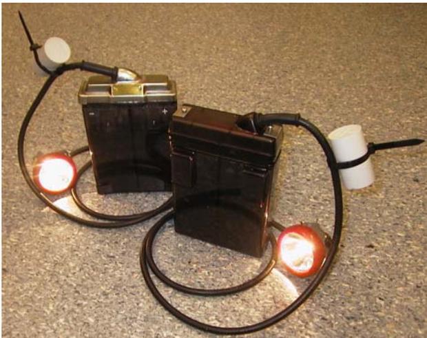
Fig. 10. Encapsulated LAMPS tag II mounted on Oldham type T2 and T4 battery cables.
