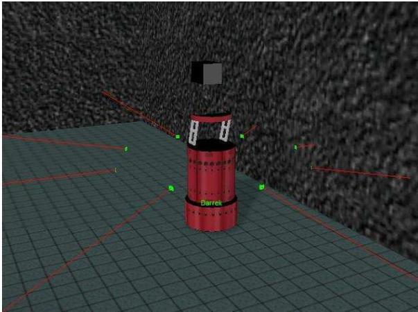
Figure 5: The B21r using its sonar sensors (each red line indicates a sonar reading length) and its camera (the black box on top of the robot) in a simulation
