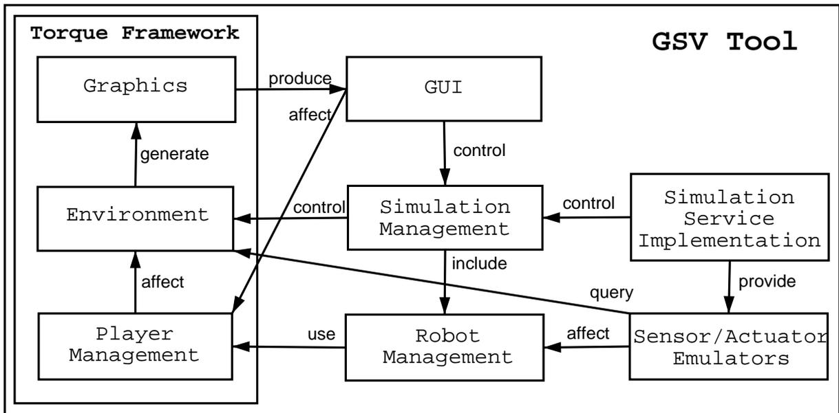
Figure 4: GSV Tool implementation and its relation with the Torque framework
