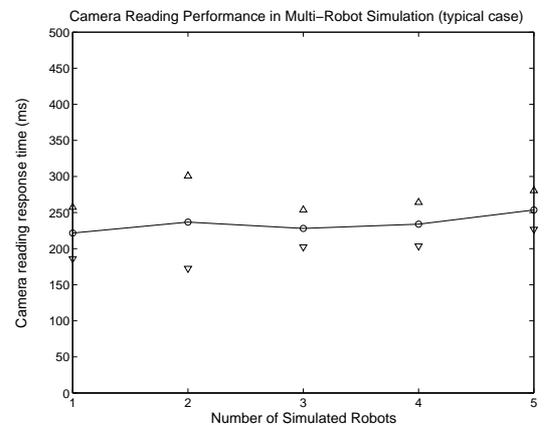
Figure 8: Camera reading response time (typical case)
