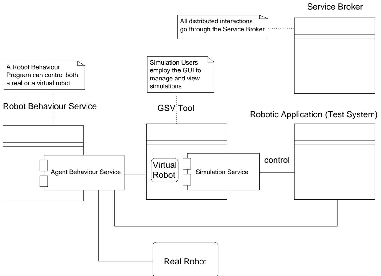
Figure 1: A GSV Tool in the Service Based Architecture. A robot application under test may control the simulation, and may use the agent behaviour service to determine robot behaviours. A real robot may also use the robot behaviour service. Where a user controls the simulation and visualisation, the GSV tool may use the robot behaviour service to determine robot actions. All distributed communications occur via the service broker (links not shown).
