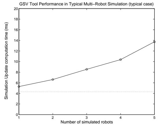
Figure 7: Effect of the number of robots on the GSV Tool performance (typical case)
