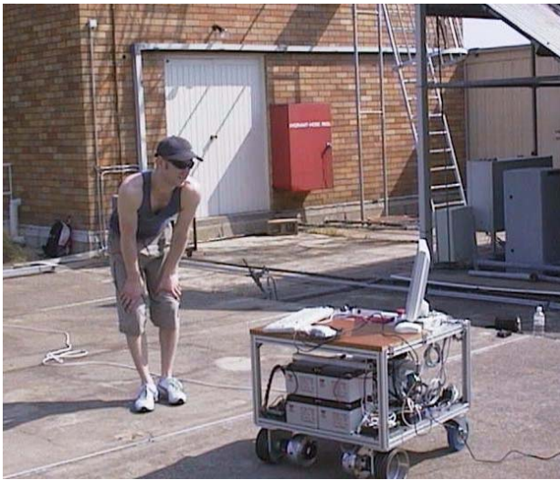
Figure 5 Autonomous mobile robot GPS test platform
