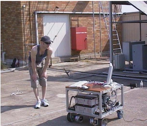
Figure 5 Autonomous mobile robot GPS test platform
