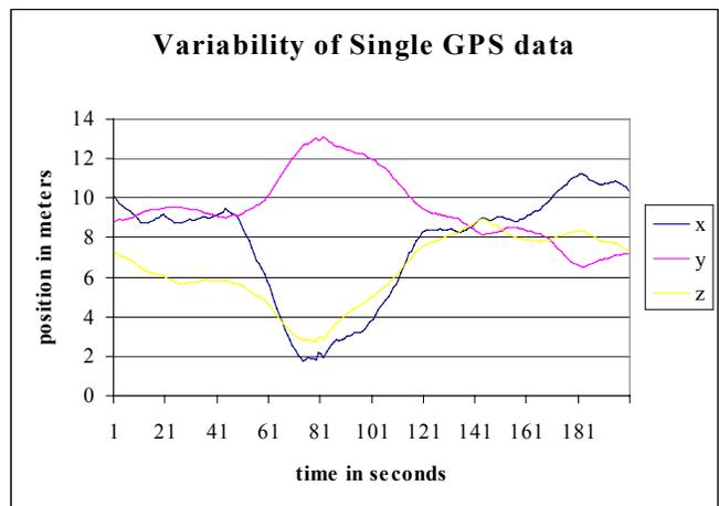
Figure 3 Short term stability of one GPS receiver
