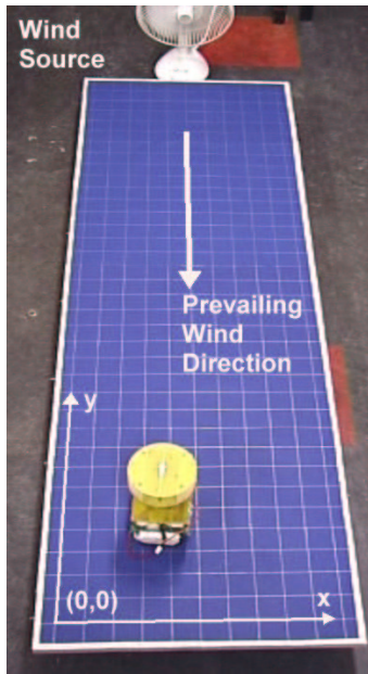
Figure 6: Simple wind seeking algorithm test area
