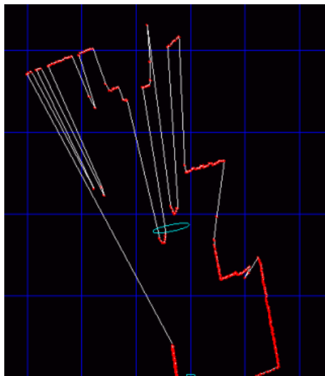
Figure 1: Raw laser scan in which two legs can be distinguished. The estimate of the person’s location is given by the cyan ellipse.
