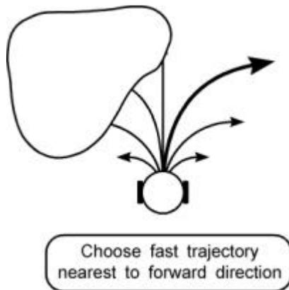
Figure 5 Object avoidance behaviour on a TVL robot.
