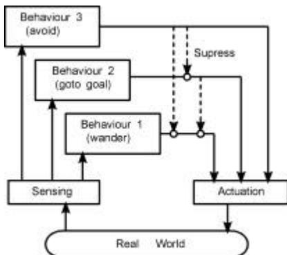
Figure 1 Subsumption architecture.
