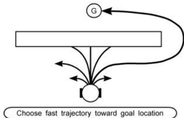
Figure 7 Goal seeking behaviour on a TVL robot.
