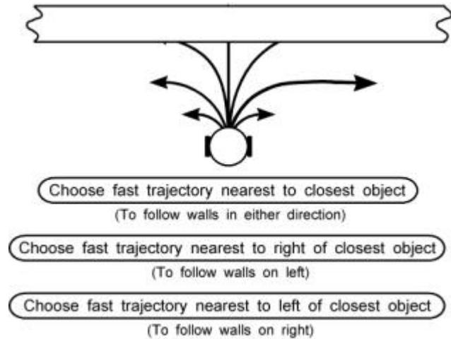
Figure 6 Wall following behaviour on a TVL robot.
