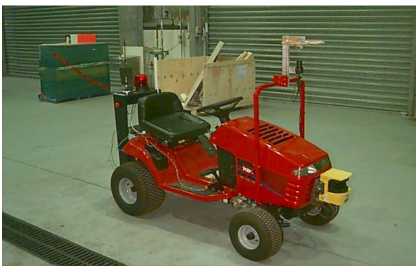
Figure 5: The experimental platform. Note the omnidirectional camera mounted over the front wheels and the box at the rear which houses the control and computer system.
