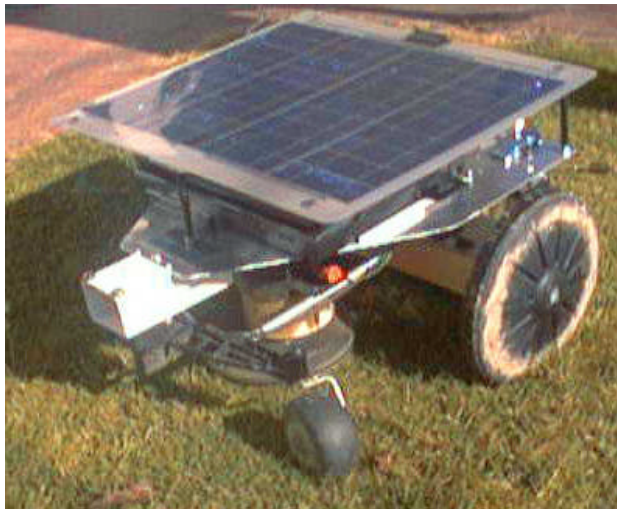
Figure 4: The Robotic Lawnmower in Operation
