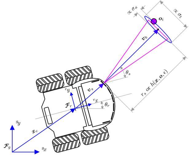
Figure 2: The Pioneer AT mobile robot detects an object  $\mathbf{o}_i$  at range  $r_s$
