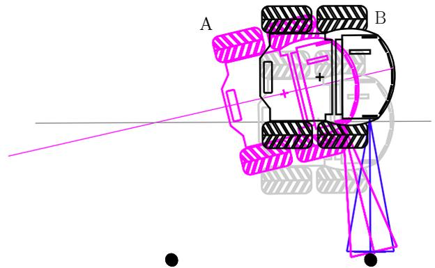
(b) The robot corrects for its apparent positional error but since it has no record of having encountered the previous object it can only conclude that it has drifted sideways.
