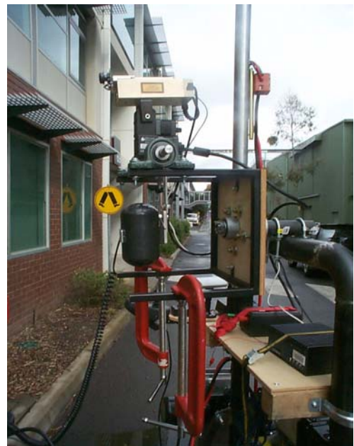
Figure 1(d) - Close Up 300m Range Scanning Laser Rangefinder (also Gyro Stabilised)
