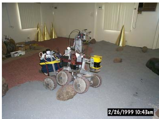
Figure 2 - Half Scale Working Marsokhod M96 Mobile Robot
