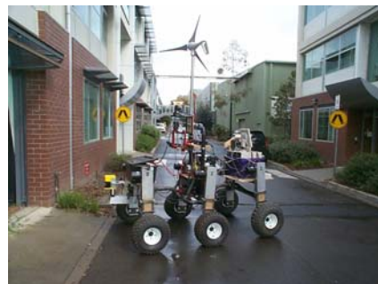
Figure 1(a) - Side View Instrumented 6WD Articulated Robot Vehicle
