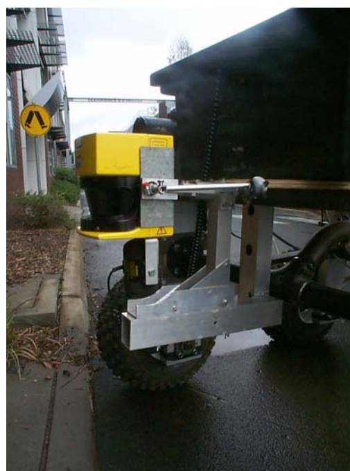
Figure 1(c) - Close Up Gyro Stabilised Sick Rangefinder
