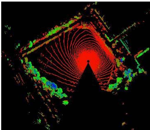
Figure 5 - Typical Long Range Laser Rangefinder Scan
