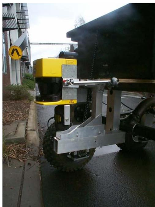
**Figure 1(c) - Close Up Gyro Stabilised Sick Rangefinder**
