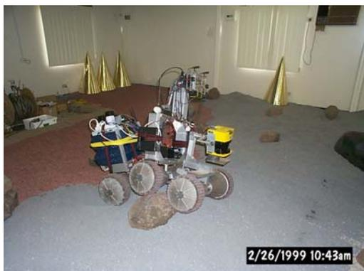
**Figure 2 - Half Scale Working Marsokhod M96 Mobile Robot**
