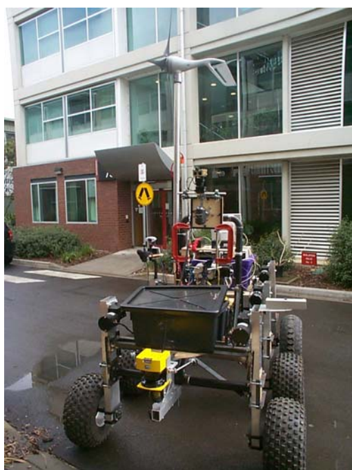
Figure 1(b) - Front View Instrumented 6WD Articulated Robot Vehicle
