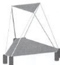
Figure 1: A schematic view of the basic Stewart platform
