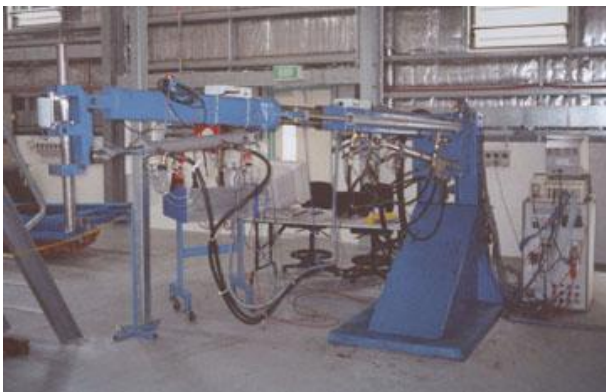
Figure 1: Experimental hydraulic robot arm.
