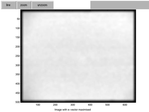
Figure 2: Intensity plot taken with polarizing film aligned with e-vector pattern, i.e. polarizing film transmission axis is at  $90^\circ$  to the solar meridian and transmission of the e-vector is a maximum. Note the relatively uniform intensity in the image.
