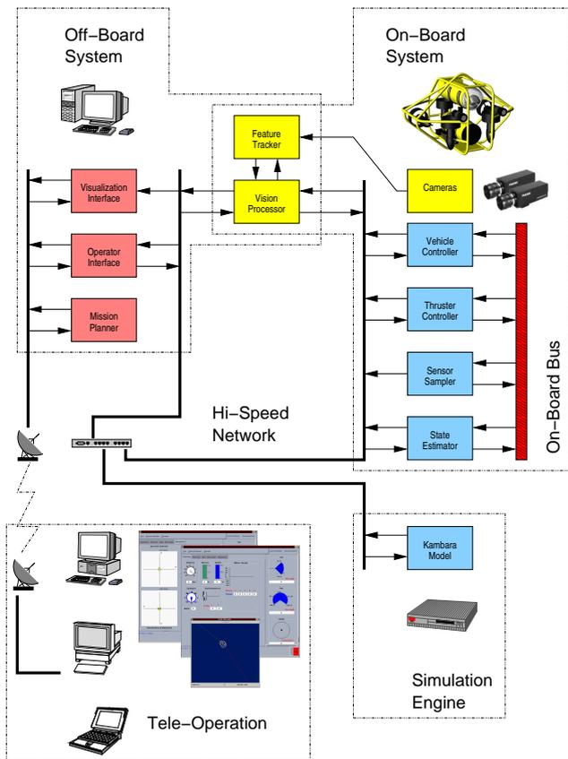
Figure 2: *Kambara*'s modular software architecture.
