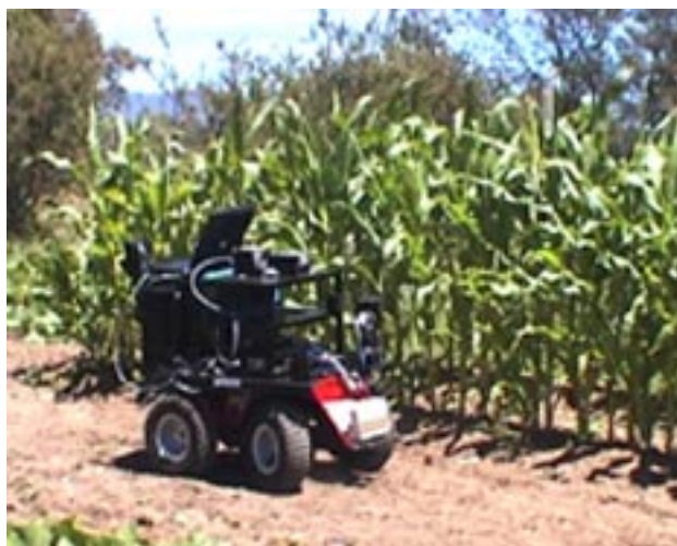
Figure 4. Titan navigating along a row of corn using a CTFM phased array ultrasonic sensor.
