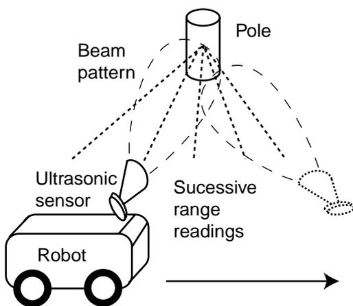
Figure 6. Sensing a simple-discontinuous landmark.
