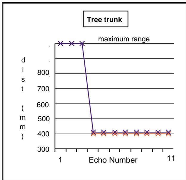
**Figure 9.** Range readings from a tree trunk, after thresholding, when the sensor scanned onto it from the left as in Figure 7 - bottom curve is start of echo, top curve is end of echo.
