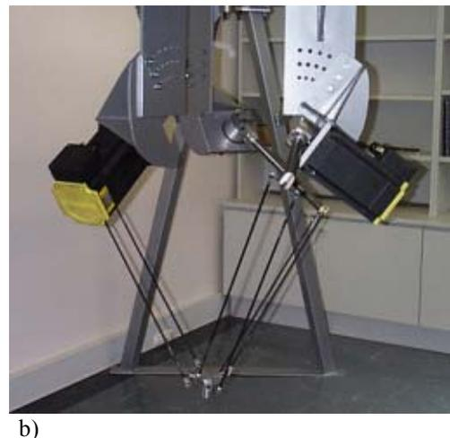
Figure 1. New University of Western Australia Robot – NUWAR a) layout; b) prototype
