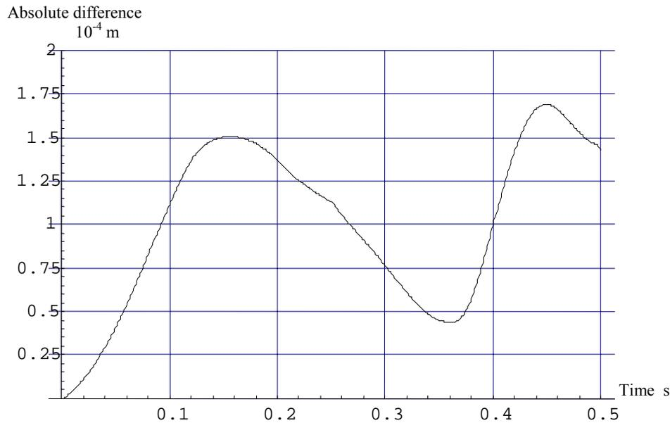
Figure 3. Results of forward dynamics calculations – the difference between the trajectory serving as input to inverse dynamics and the result of forward dynamics calculations using torque histories of Figure 2.
