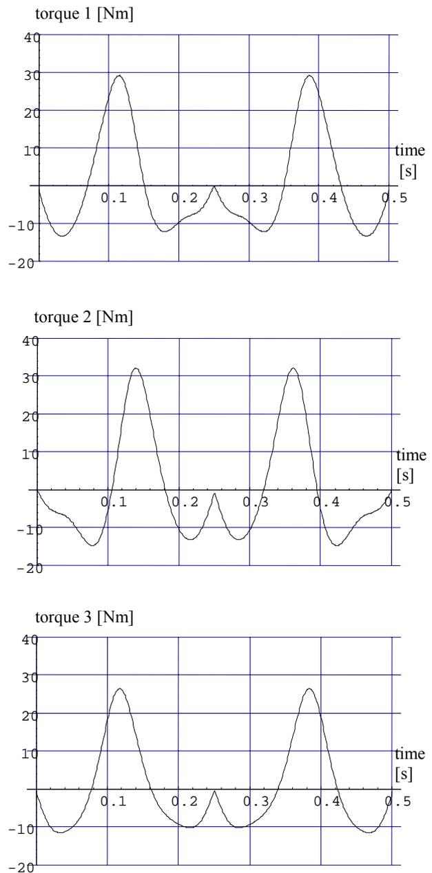
Figure 2. Results of inverse dynamics calculations – time histories of motor torques required to produce the elliptical trajectory described above.
