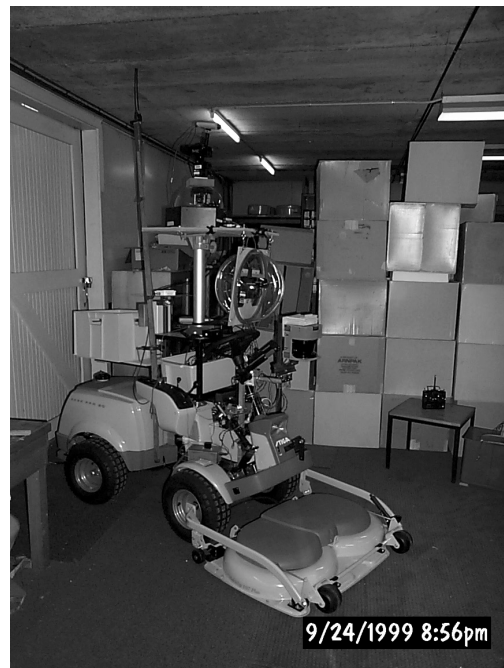
Figure 1(a). Stiga Pro. 20 Mower — Fully Instrumented
