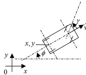
Figure 2 State and control of the vehicle.
