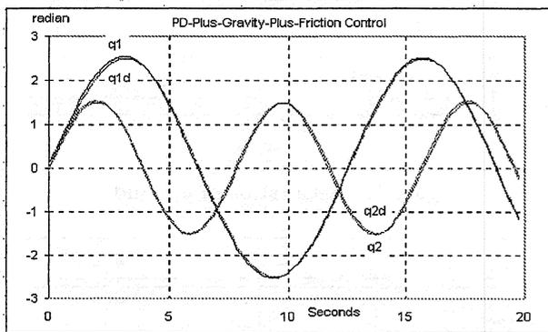
Figure 16: PDGF tracking control
