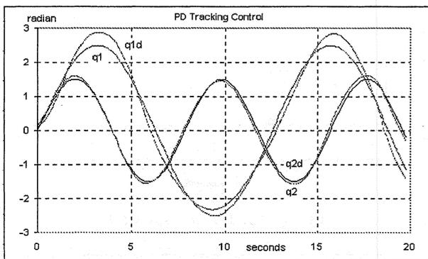
Figure 15: PD tracking control
